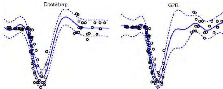
Fig. 1. Toy regression example in 1-D: we predict the y -values from the x -values in a synthetic signal generated by a combination of Gaussian bumps. We show the predictive variance or confidence interval estimates via bootstrap variance estimates (left), and Gaussian process regression (right).
