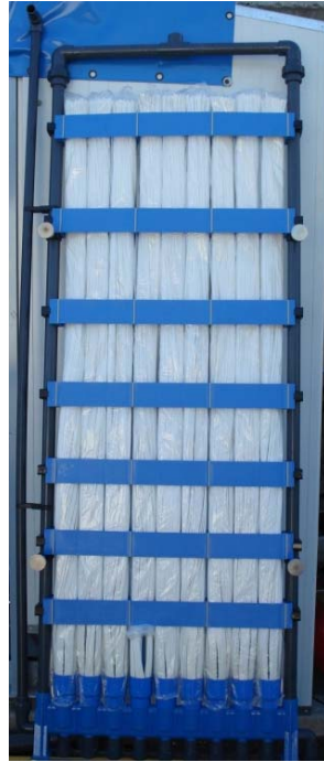
Figura 13. Módulos de membranas comerciales PURON®, Koch Membrane Systems PUR-PSH 31HD.
