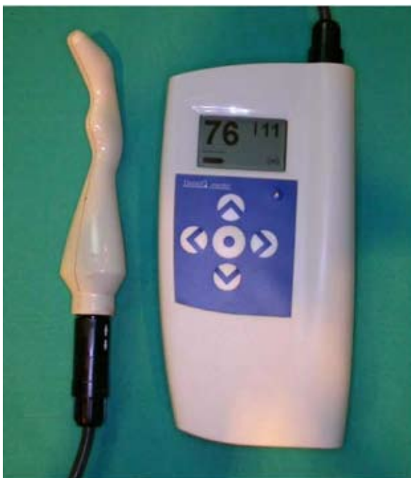
Fig. 3. An Osstell transducer
