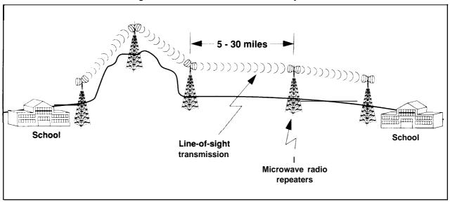
Figure Microwave Communication System
