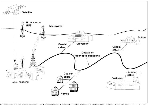
Figure 3-6--Cable Television Distribution System
