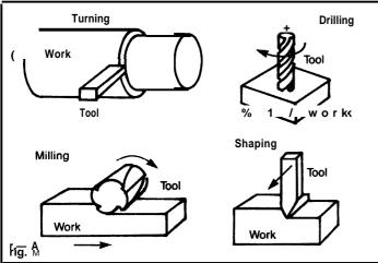
Figure 4.— Fundamental Operations in Metalworking
