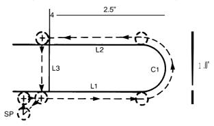
The path of the center of the cutter is shown as t moves about the perimeter of the part.
