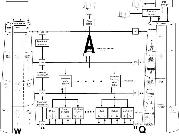
Figure 10.—NBS Scheme for Distributed Factory Control
