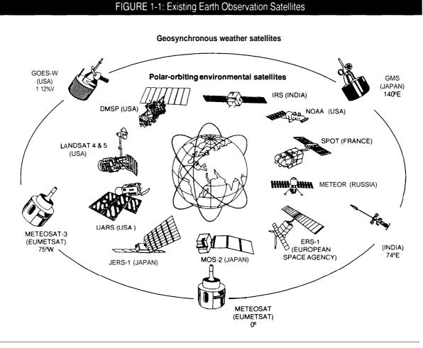
NOTE: Several countries operate satellites to monitor Earth and to collect environmental data. This figure depicts most of the satellites that are either n geosynchronous or polar/near-polar orbits.
