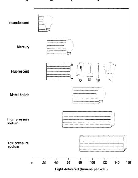
Figure 4-5-Energy Efficiency of Various Light Sources
