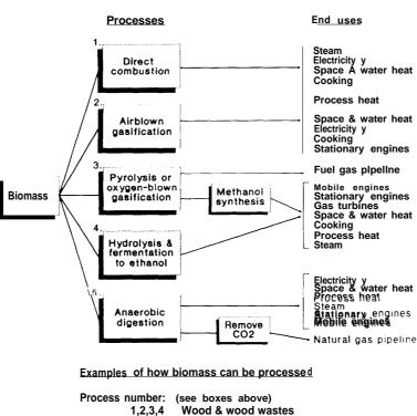
Figure 3A-I—Alternative Methods of Using Biomass Energy
