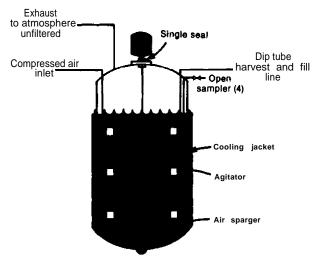
Figure 17-1 .—Features of Standard Fermenter
