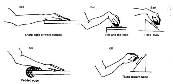
Jigs should be located and oriented so that parts can be assembled without flexing the wrist.
