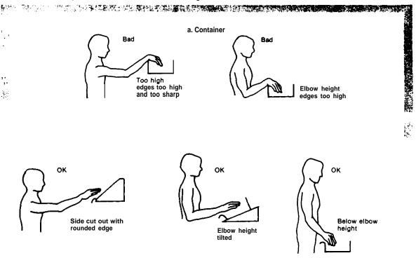
Containers should be designed so that workers can reach all locations without flexing their wrist. All edges that come into contact with the worker should be well rounded.
