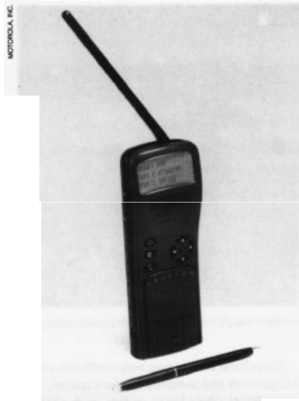
Dual-mode portable telephones, such as this prototype from Iridium, will first attempt to connect to a local cellular system. If no system can be accessed, the telephone will then use the satellite system to complete the call.
