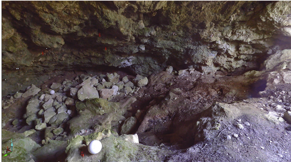
Fig. 5. One of the point clouds captured showing the interior of Pastora Cave in RGB. Point cloud composed of approximately 28,000,000 points.
