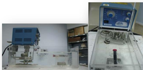
Figure 32. Water phantom with the blood sample submerged
