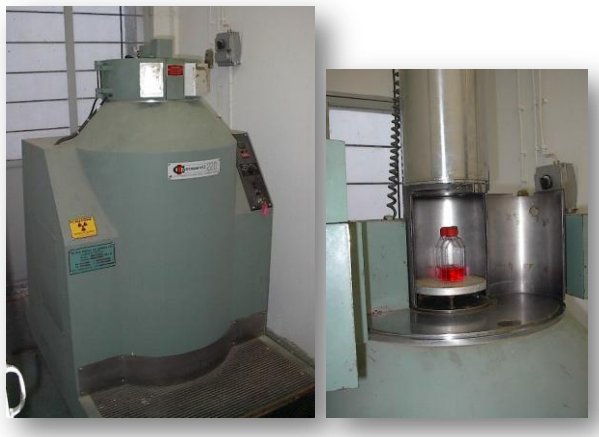
Figure 38. Flasks in the Gamma Cell 220 irradiator (Institute of Radioisotopes & Radiodiagnostic Products, National Center for Scientific Research, NCSR “Demokritos”, Athens).
