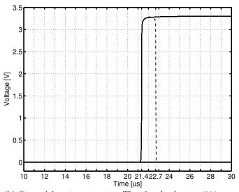
(b) Starved inverter outputs. The signals close to Vdd correspond to the cells with the largest differential input values. The signals close to 0 V correspond to the cells with the lowest differential inputs. The dashed line corresponds to cell 0.
