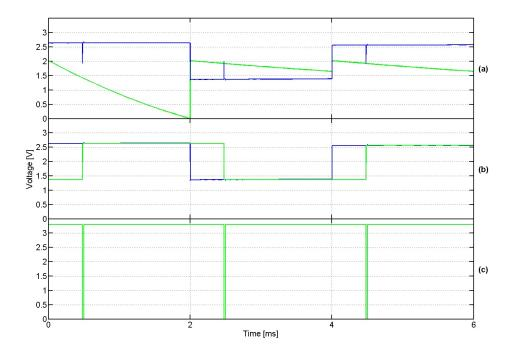
Figure 3.3. Simulations of the photocircuit operation. Voltage signals at nodes (a)Vphd (green) and Vpresent (blue), (b) Vpresent (blue) and Vprevious (green), and (c) WTAfeedback. Integration time is 2 ms, low level pulse width of WTAfeedback is 20  $\mu$ s, Vreset=2 V, Vflr=2.3 V, Vbufflow=1.8 V and Vbuffhigh=1.6 V.
