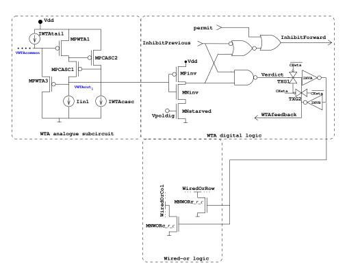
**Figure 3.12.** WTA analogue/digital circuit for single winner selection. Subscript notation  $_{-r_{-}c}$  indicates row r and column c.
