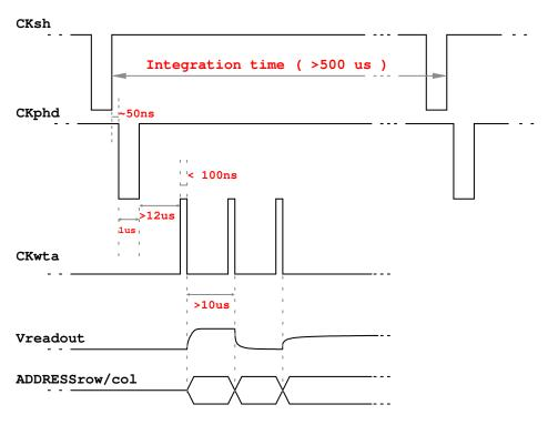
Figure 4.3. SCD sensor synchronization. In this example only 3 pixels per integration time are transmitted out of the sensor.
