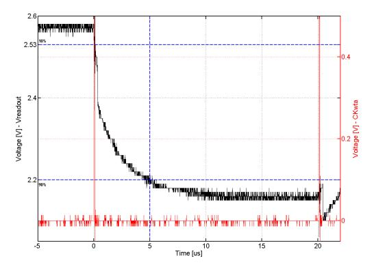
Figure 4.4. Gray level output signal (black line, node Vreadout) synchronized with CKwta clock (red line).
