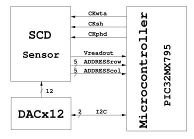
Figure 4.1. SCD camera and processing system. Vreadout is the analogue grey level signal (see Fig. 3.2), ADDRESSrow and ADDRESScol are the row and column address bus, respectively. CKsh and CKphd are the photocircuit clock signals (see Fig. 3.2), and CKwta is the clock signal for the WTA digital logic (see Fig. 3.12).
