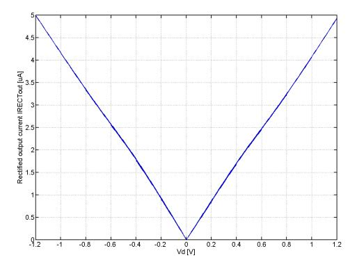
$Id_{Nin}$  is mirrored by MPRECT2-3 transistors, in both cases, IRECTmirror is positive [80].
