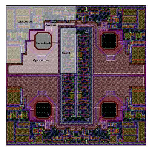
Figure 3.18. Basic 4-pixel reproducible layout unit. The size of one single pixel is  $55\mu m \ge 55\mu m$ .
