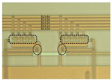
(b) Microphotograph of the address-codifier transistors of rows 30 and 31 (black dashed rectangles) together with pull-up transistors MPWORr\_30-31 (black dashed ellipses).
