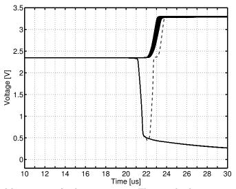
(a)  $\mathsf{VWTAout}_k$ , for k = 0...1023. The signals close to Vdd correspond to the cells with the lowest differential input values. The signals below 0.5 V correspond to the cells with the largest differential inputs. The dashed line corresponds to cell 0.
