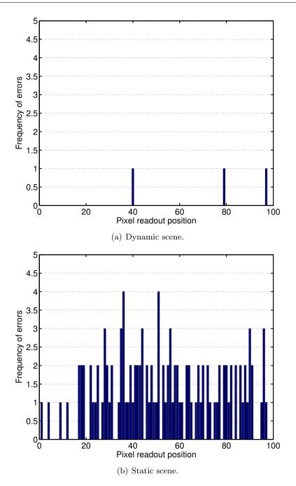
Figure 4.8. Histogram of WTA failures (WTA stage not being able to choose a winner) as a function of the position in the readout sequence for two different types of scenes: dynamic and static.
