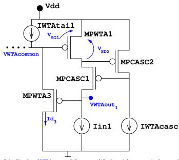
(b) Single WTA amplifier modified with a gain-boosted regulated-cascode stage.
