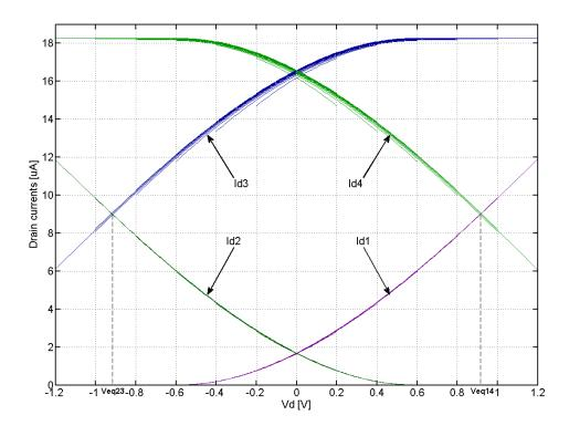
Figure 3.7. Drain current for transistors MNOTA1-4. For every transistor, a total of 11 curves are plotted for different Vc values ranging from 1.4 V to 2.6 V with a 0.1 V step. Simulations were performed with VOTApol=0.9 V.
