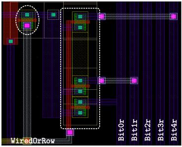
(a) Address-codifier transistors of row 19 (white dashed rectangle) together with pull-up transistor MPWORr\_19 (white dashed ellipse).
