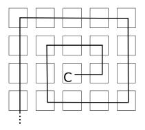
Figure 3.24. Proposal for a different topology for the inhibiting signal path. The small squares represent the pixels in the matrix. The pixel labelled with letter C is in the centre of the matrix. Its precise address depends on the matrix size.
