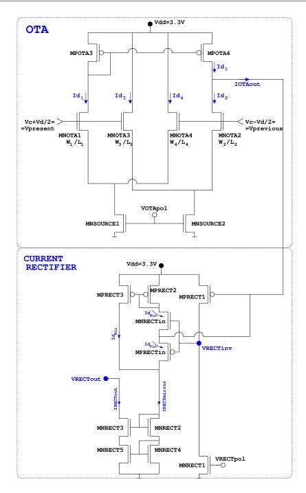
Figure 3.6. Wide input range OTA and rectifier subcircuits.
