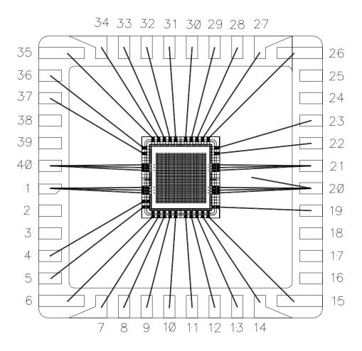
Figure 3.21. Bonding diagram.
