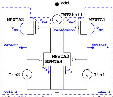
(a) Basic WTA circuit with two competing input currents, Iin1 and Iin2.
