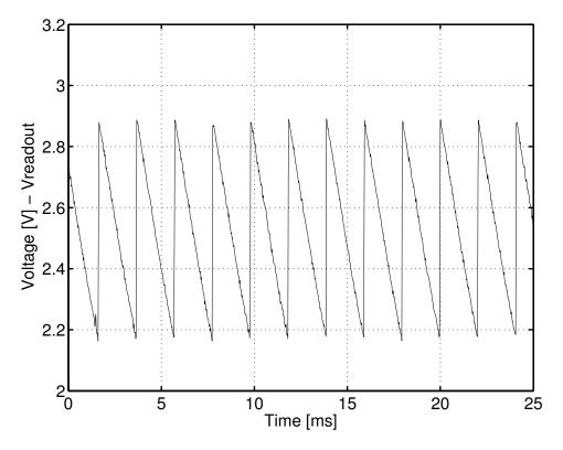
Figure 4.11. Oscilloscope capture of the Vreadout noise during temporal noise measurements.
