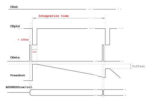
Figure 4.9. Time diagram for noise measurements. CKsh = 0 V.
