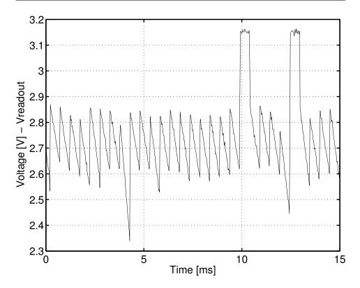
Figure 4.10. Oscilloscope capture of the Vreadout noise during FPN measurements. Integration time is 500  $\mu$ s.
