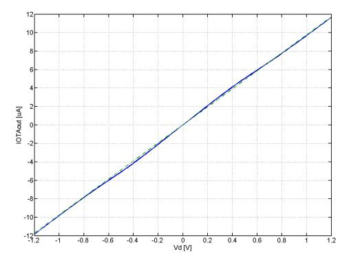
Figure 3.8. OTA's output current IOTAout (continuous blue curves). A total of 11 curves are plotted for different Vc values ranging from 1.4 V to 2.6 V with a 0.1 V step. Simulations were performed with VOTApol=0.9 V. Dashed-dotted green curve is a straight line with slope  $12/1.23 \ \mu A/V$ .
