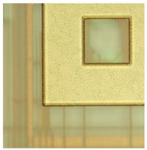
(b) Detail of the fourth metal layer covering the whole pixel matrix. Only the photodiodes are exposed to incident light.
