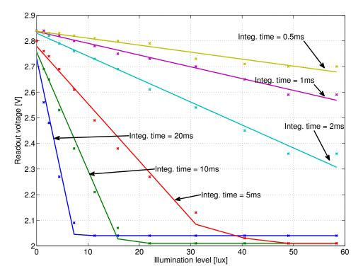
Figure 4.5. Sensor output voltage against light intensity for different integration times. Continuous curves are the linear regression fitting of data in Table 4.2. The crosses (x) correspond to the raw data of Table 4.2.
