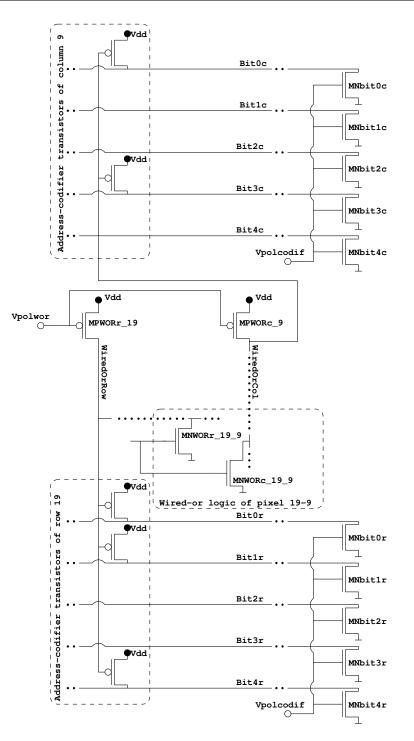
Figure 3.15. Wired-or and address-codifier transistors of the pixel in row 19 and column 9.
