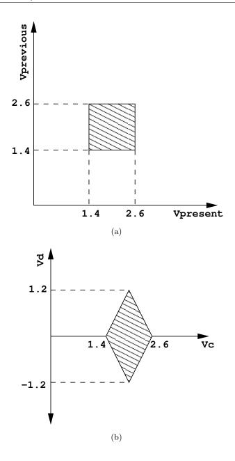
Figure 3.4. Streaked areas represent the OTA's input voltage range expressed in (a) Vpresent-Vprevious, and in (b) common mode (Vc)-differential mode (Vd) values.
