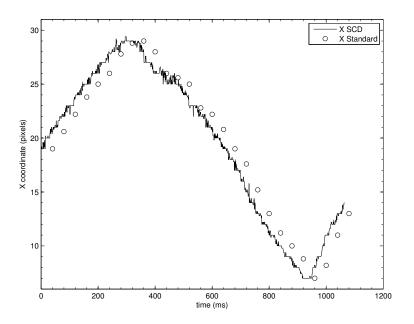
Figure 4.13. x coordinate of the object oscillating at 0.8 Hz
