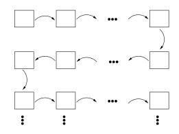
Figure 3.13. Propagation path for WTA digital inhibition signals.
