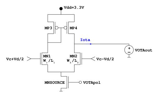
Figure 3.5. Narrow input range OTA.  $W_1/L_1$  and  $W_2/L_2$  are the width/length ratio for transistors MN1 and MN2 respectively.
