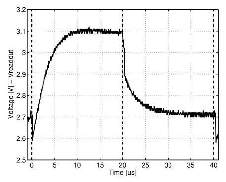
Figure 4.7. Oscilloscope trace of the readout signal reaching values higher than 3.0 V. CKwta period is 20  $\mu$ s. Vertical dashed lines show winner selection timing.
