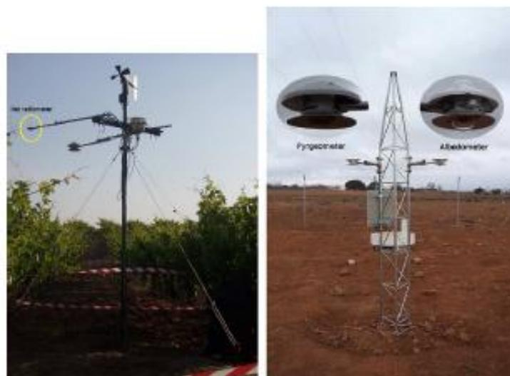
Fig. 3. (left) Net radiometer used to measure net radiation at surface in the FESEBAV experiment and (right) radiometer used at WAS that measure net radiation components separately (downwelling and reflected shortwave radiation, downwelling and upwelling longwave radiation).
