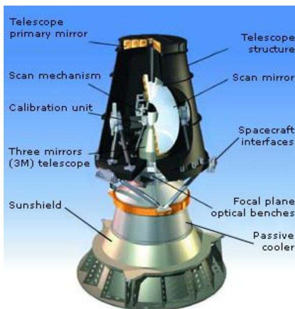
**Figura I.8** - Detalles del sensor SEVIRI (*Spinning Enhanced Visible and Infrared Imager*)
