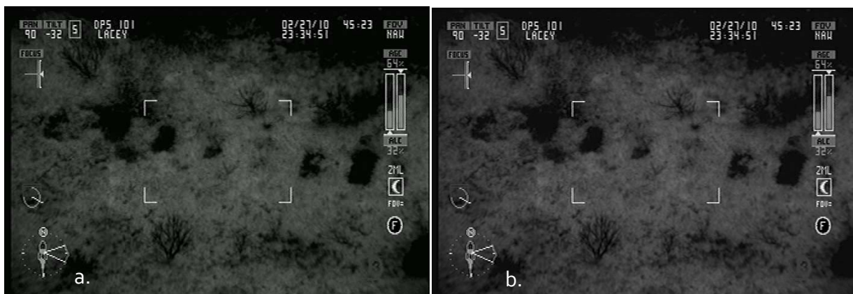
Figure 7. The three-band composite (a) and actual grayscale (b) versions of image 6r11 (unrectified). Contrast between image features is less pronounced in (b).
