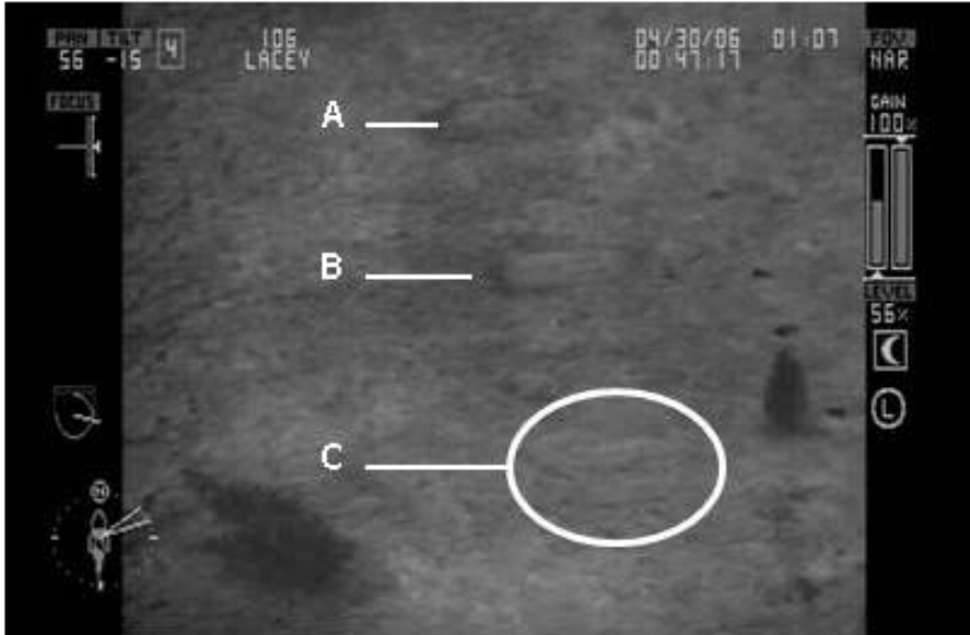
Figure 1. Thermal image of the preliminary test site at 500 feet, April 2006 flight. Darker features are warm. Scale is approximately 1:200. The outlines of units A (0.5 meters) and B (1.0 meter) are readily observed. Unit C (1.5 meters) appears faint. Poor discrimination was likely due to excessive rainfall.
