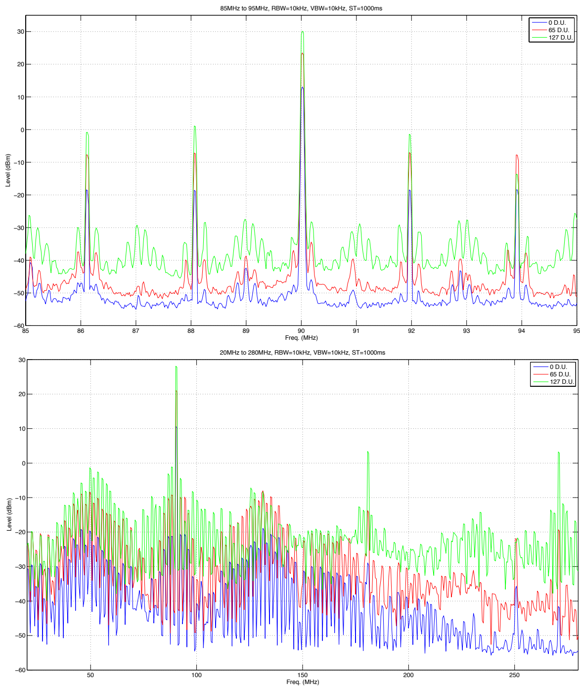
Figure 5.3. RF output spectra of the DDS driver when generating a 90MHz single tone, at three different power settings (minimum, medium, and maximum), shown in the range from 85MHz to 95MHz ( top ) and from 20MHz to 280MHz ( bottom ).
