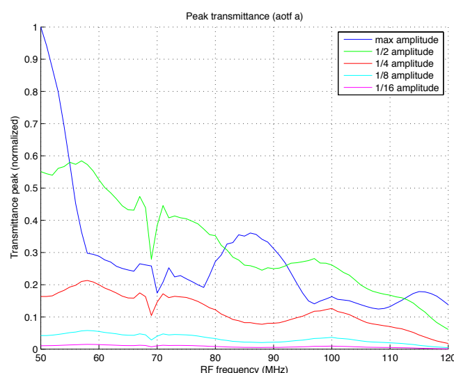
Figure 7.14. Peak transmittance of the ATFS instrument for the first set of measurements.
