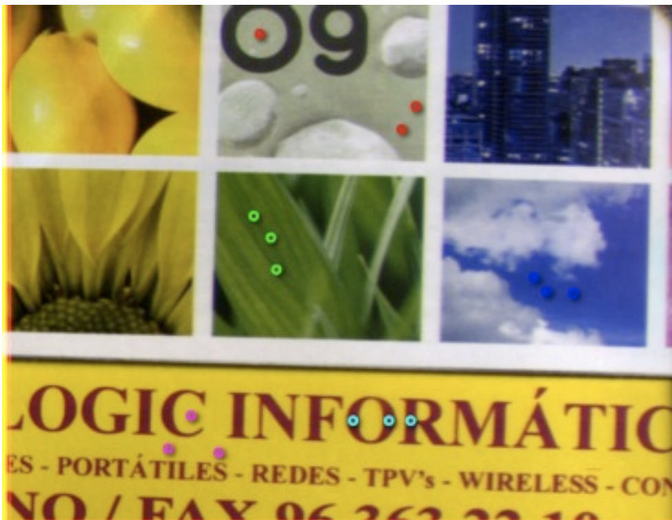
Figure 8.14. RGB image of the calendar target taken with the ATFS system. Circled areas show the areas used to plot the spectral reflectance.
