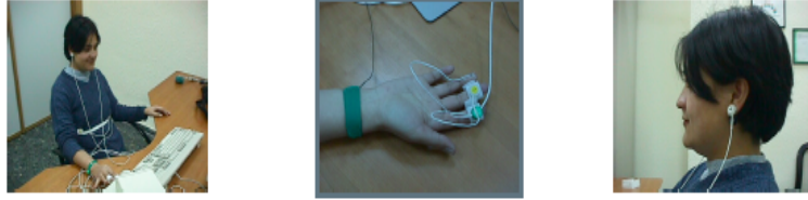
Fig. 3. Different electromyograph and polygraph electrode positions.
