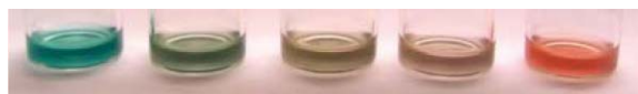
Fig. 4 Photograph of a suspension of solid P1-MS in contact with aqueous extracts of gilthead bream ( S. aurata ) at pH 10 with increasing amounts of histamine after 30 min of reaction at 50 °C. From left to right: C_{\text{histamine}} = 0, 3.75 \times 10^{-3}, 6.25 \times 10^{-3}, 1.25 \times 10^{-2} and 2.50 \times 10^{-2} M.
