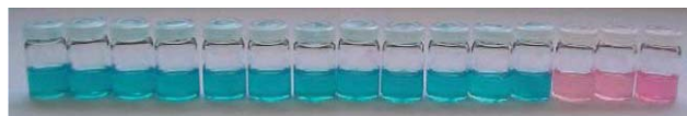
Fig. 1 Photograph showing the colour change in P1-MS in the presence of amino acids and biogenic amines. From left to right: no guest, glycine, valine, leucine, phenylalanine, proline, tyrosine, arginine, tryptophan, cysteine, lysine, histidine, histamine, putrescine and cadaverine. The final solids filtered and suspended in ethylene glycol are shown.
