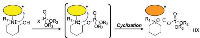
Fig. 3 General scheme of PET indicator molecules for the fluorogenic detection of nerve agents.
