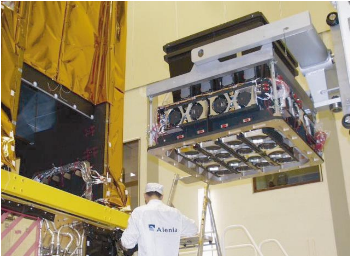
Fig. 1. The IBIS Detector Unit during final mechanical integration on the S/C at ESTEC: in the picture are visible the Veto BGO modules, the Hopper structure and the Payload Module with the open Detector housing; the internal black wall is part of the Lead Passive Shield extending up to the Coded Mask.
