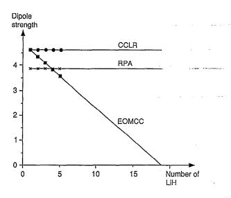
FIG. 1. The dipole strength as a function of the number of noninteracting LiH systems within the CCLR, RPA, and EOMCC approaches. Calculations have explicitly been carried out for up to five systems.
