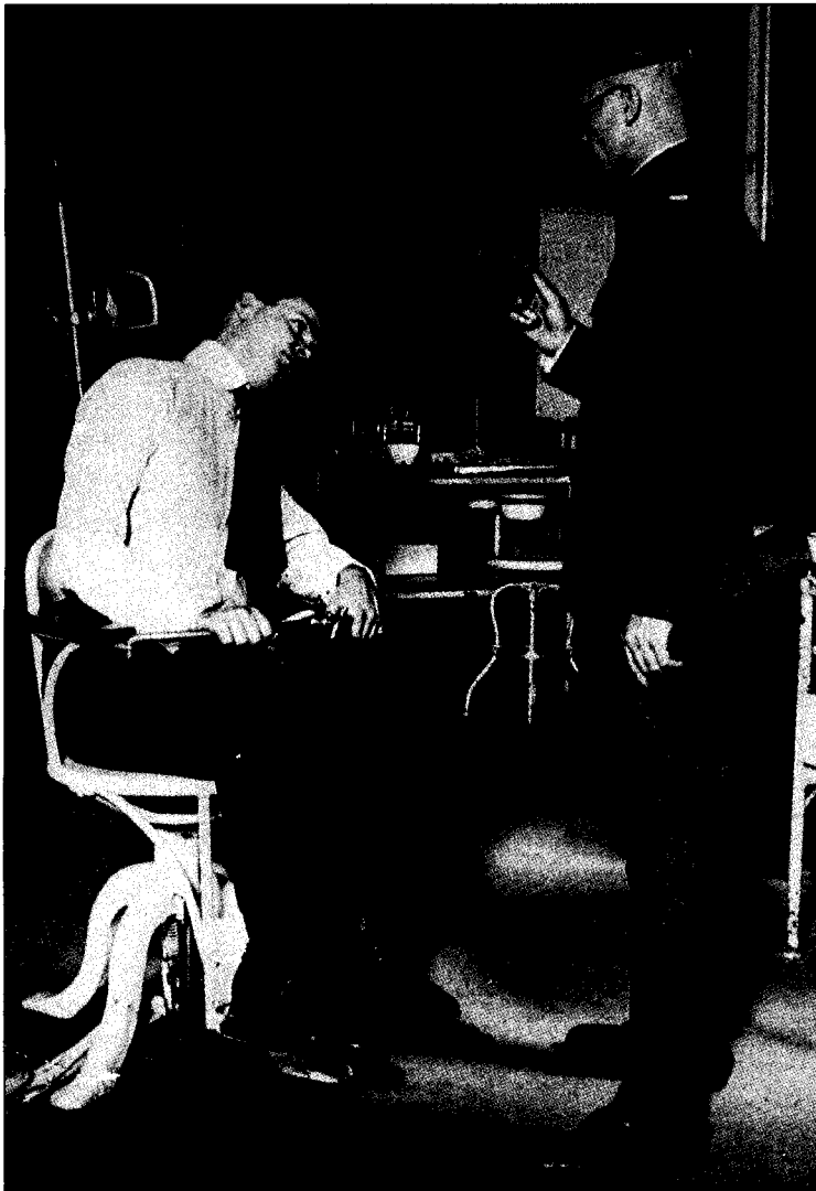
Barany Chair used in early aviation medicine to test pilots orientation ability.
