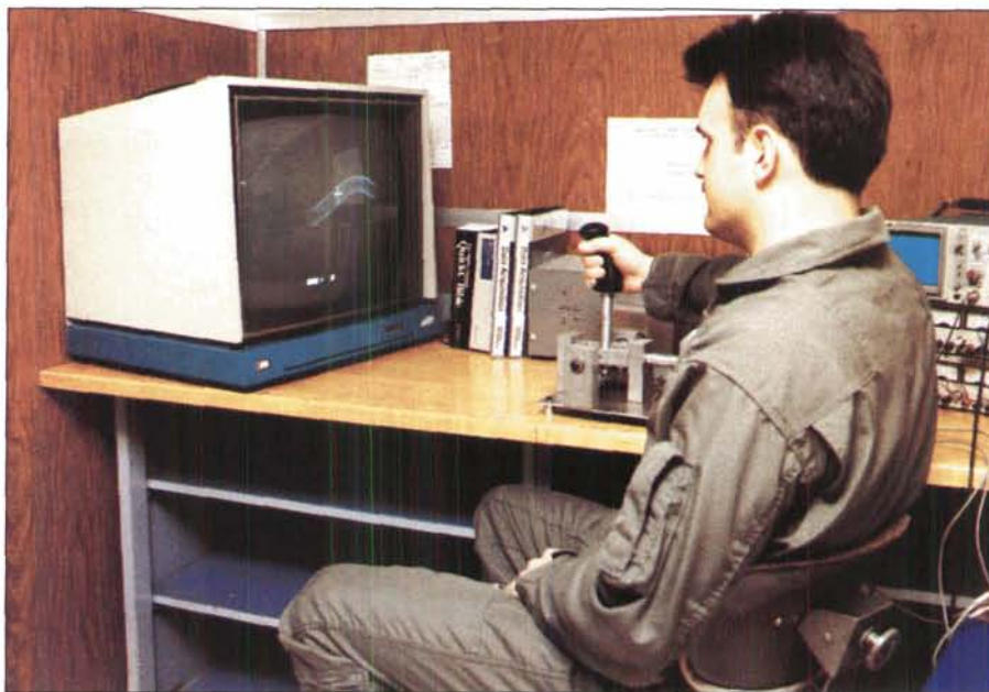
Force reflection provides smoother tracking during random arm movements.
