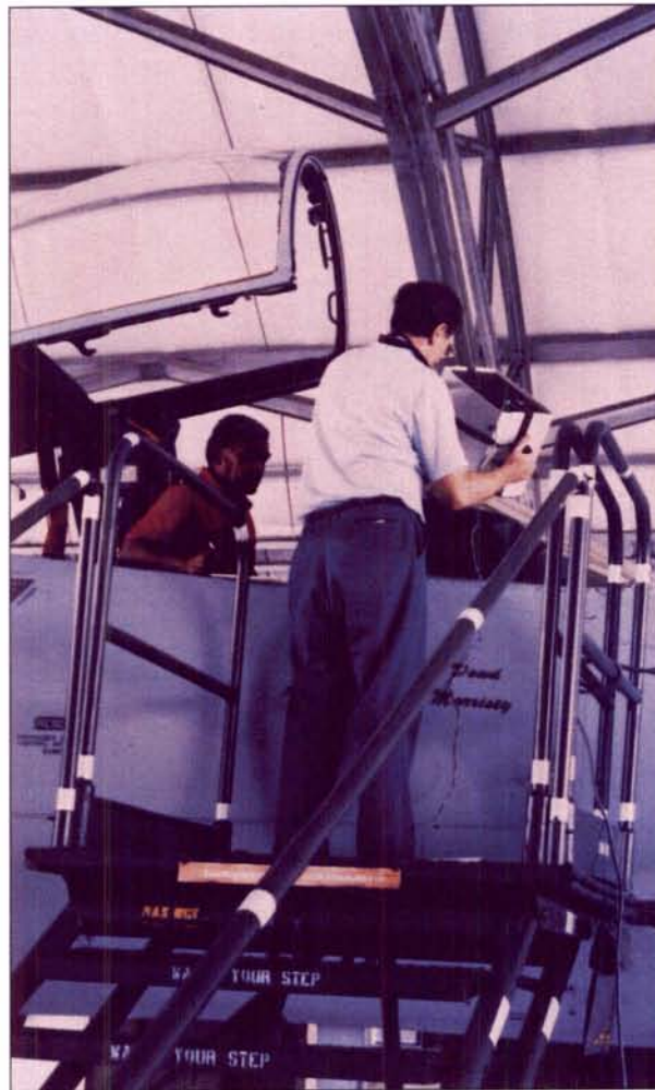
Haze-o-Meter II being used to measure F-15 canopy during device field test at Eglin AFB FL.
