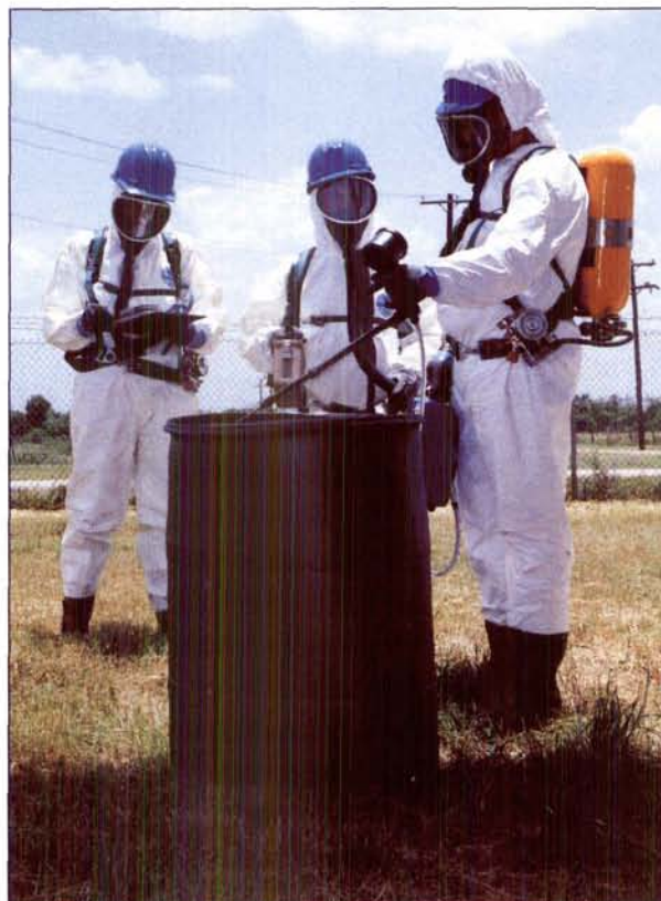
Bioenvironmental engineers sampling a drum before a hazardous waste sample is obtained.
