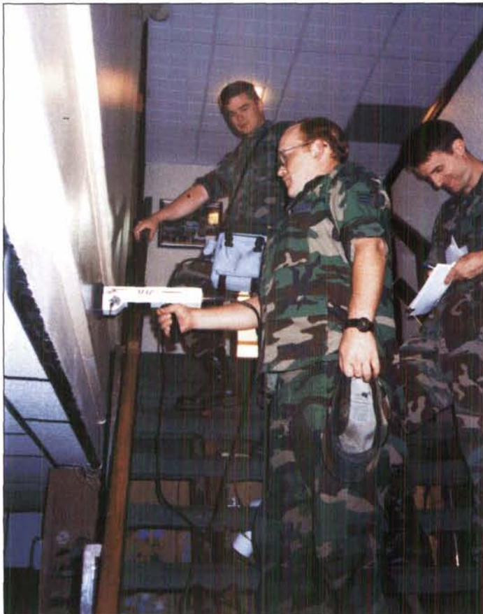
X-ray fluorescence monitoring for lead based paint.
