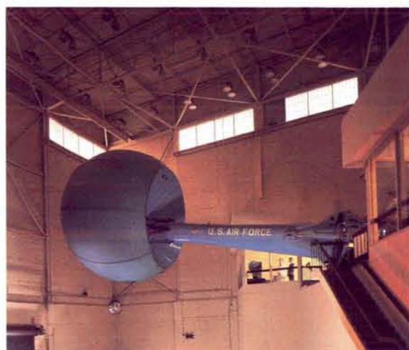
The LAMARS' large amplitude motion capabilities provide vital pilot cueing, essential in aircraft flying qualities research.
