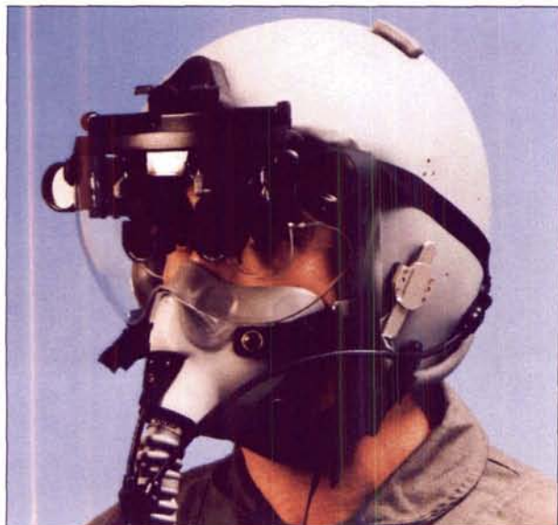
New NVG design fits underneath issue helmet and provides improved visual acuity.
