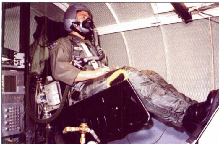
Advanced +Gz-protection, illustrating the newly introduced pressure breathing system (COMBAT EDGE) and the advanced technology anti-G suit (ATAGS).
