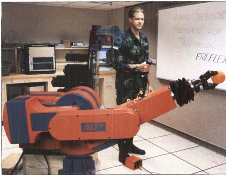
Operator remotely controls strength with which robot picks up object.
