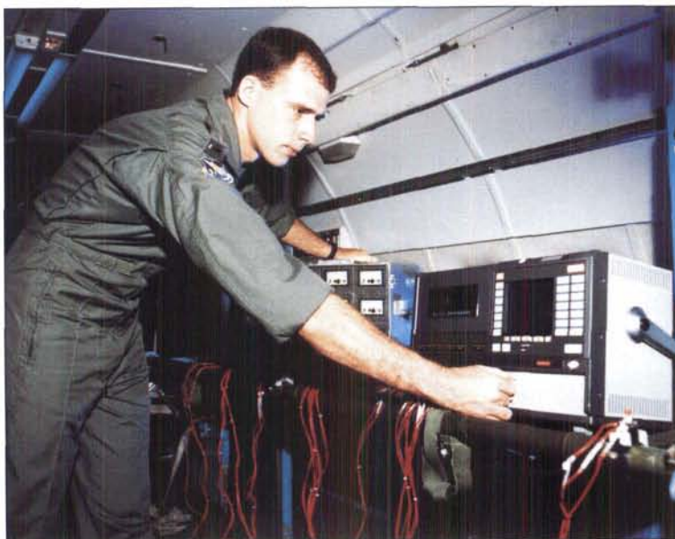
A vibration study is conducted on a C-9A to validate test criteria for air evacuation medical equipment.
