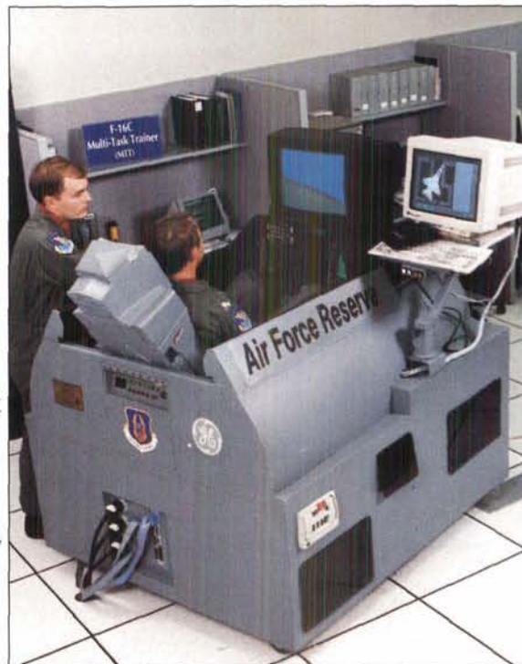
The F-16C Multitask Trainer provides high fidelity training within a portable platform costing only a fraction of existing trainers.
