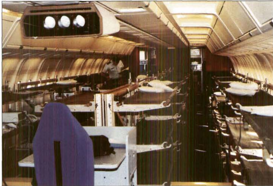
Installation of these shipsets in existing commercial B-767s will enhance our wartime capability to evacuate the injured.
