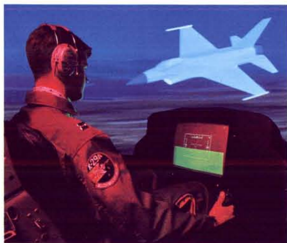
The MS-1 and LAMARS simulators utilize an over-the-shoulder video camera to record the pilots' movements and reactions.
