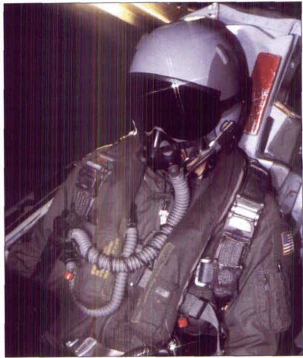
Equipped with COMBAT EDGE, pilots can tolerate greater levels of "G" force.
