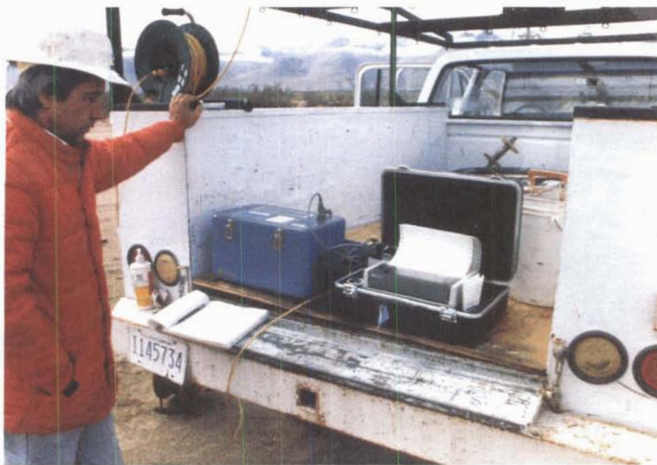
Figure 6. Pneumatic slug testing on well BR-6 (2-11-92). Pressuring the well (upper). Logging water level recovery (lower). The blue box is the data logger and the field printer is in the black, foam padded suitcase.
