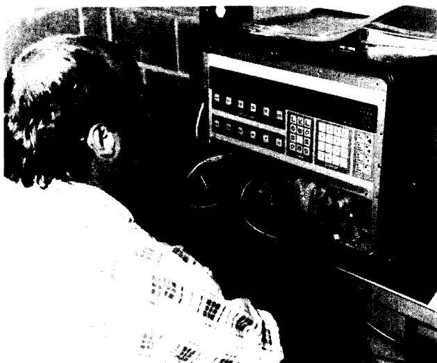
The Vaisala Mini-Rawinsonde System (MRS) receiver located in Building 279 collects weather data from balloons traveling up to 100,000 feet.
