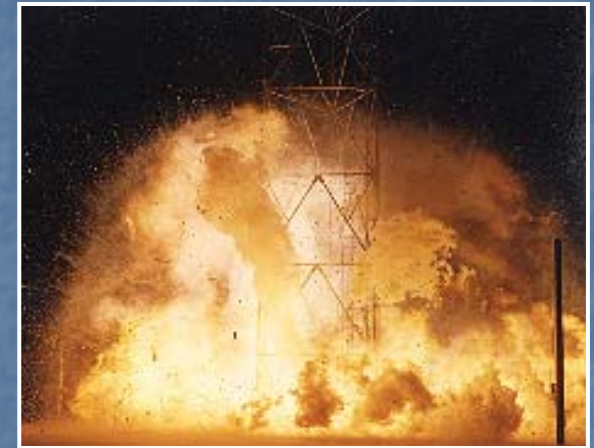
Tank Drop Test -- Explosion of 2,200 lb. LOX/LH2
