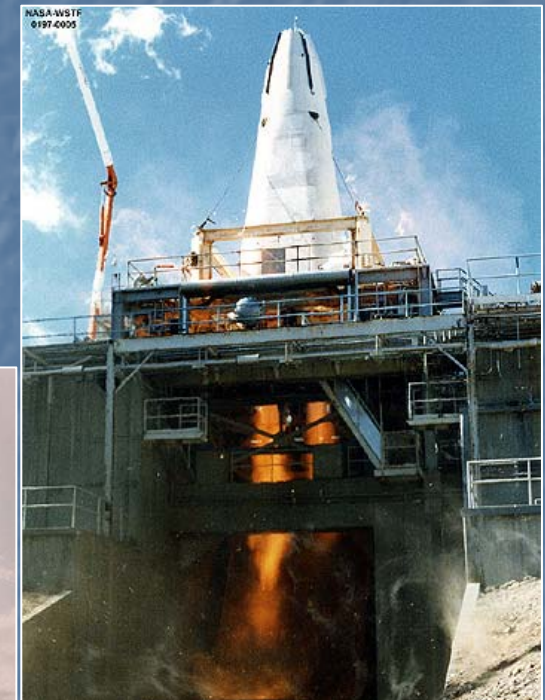
Static firing of DC-X with 4 LOX/Hydrogen RL10-A5 Engines
