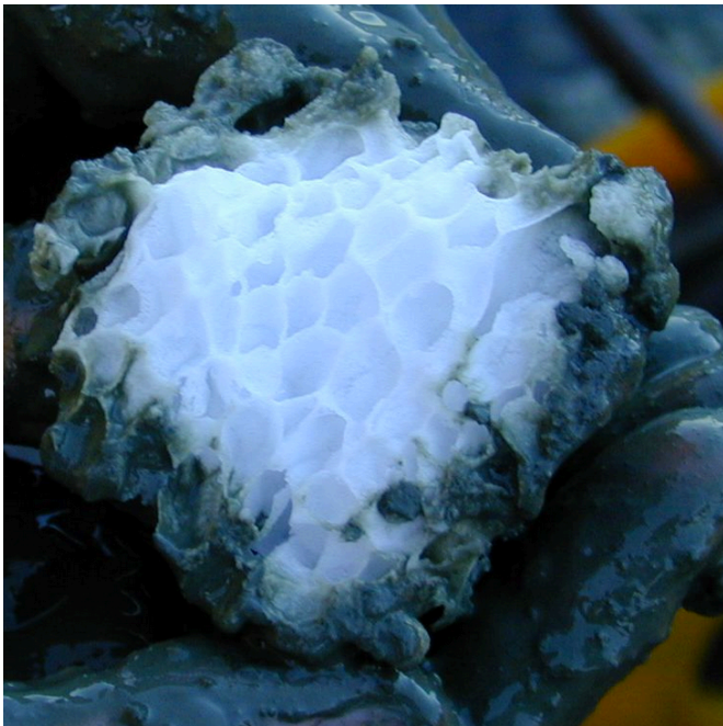
Figure 2: This cross section of a methane hydrate reveals the structural differences between hydrates and normal ice. This sample was taken from a subduction zone off the coast of Oregon. (The Guardian, 2015)
