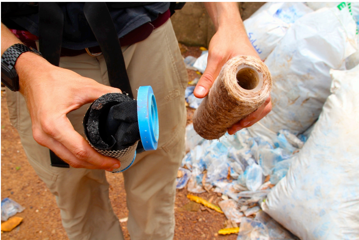
Exhausted carbon filter (left) and yarn filter (right)
