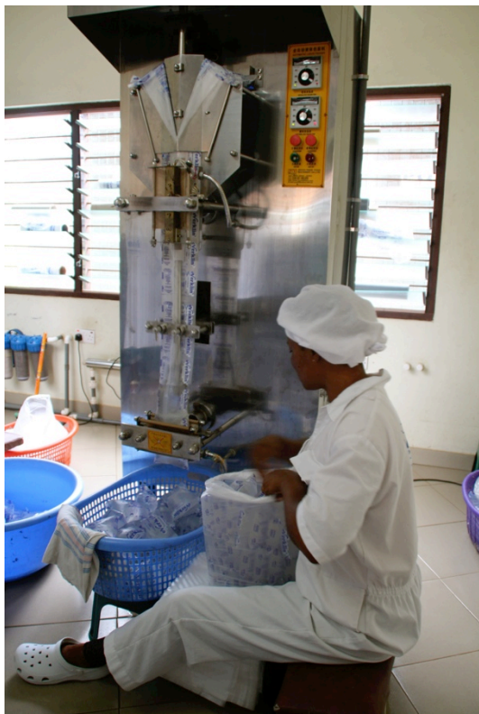
A sachet machine operator monitoring production and bagging newly made sachets
