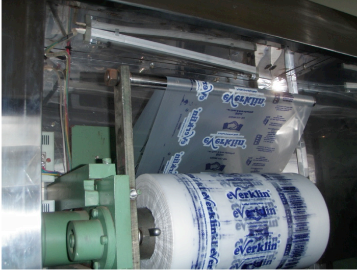
The back of a sachet machine – the roll feeds through the front of the machine, first passing under a UV light
