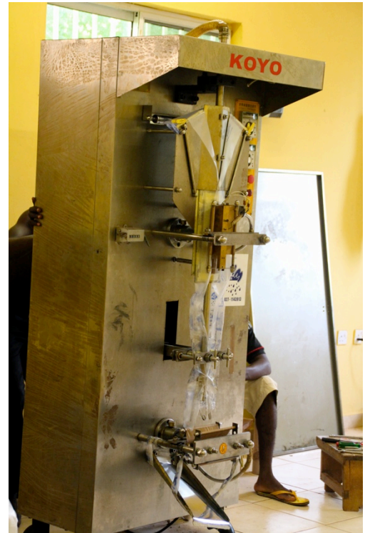
A typical “Koyo” brand sachet production machine
