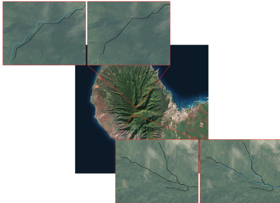
Figure 13. Evidence of currently flowing streams while determining Method 1 stream network cell-threshold. Streams on satellite basemap are interpreted as the faint white lines that flow through stream channels, which are then traced with blue lines to clearly visualize. Black lines are the stream network created with a 3162 cell-threshold ( x=3.5 ).
