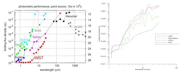
**Figure 6.2:** Limiting sensitivity plots in Janskys (Jy). Left: A collection of sensitivity values (http://www.stsci.edu/jwst/science/sensitivity) Right: Modeled values for our four idealized telescopes. The Keck and SOFIA in reality will be far worse than this.
