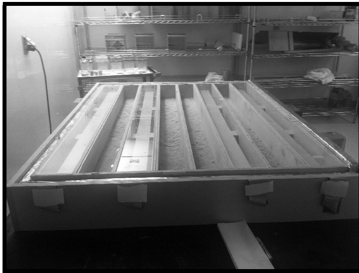
Figure 3. Thermal gradient used in experiments consisting of eight lanes, warmest end closest in picture
