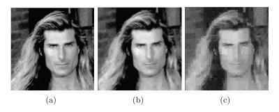
Figure 3. (a) Original  $256 \times 256$  Fabio image corrupted with Gaussian noise and its reconstruction from 20% randomly selected Fourier coefficients using (b) total variation minimization and (c)  $\ell_1$ -minimization of its bivariate Haar coefficients. Original image (a) used with the kind permission of Fabio, Inc., Santa Monica, CA.
