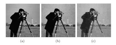
Figure 2. (a) Original  $256 \times 256$  cameraman image and its reconstruction from 20% randomly selected Fourier coefficients using (b) total variation minimization and (c)  $\ell_1$ -minimization of its bivariate Haar coefficients.
