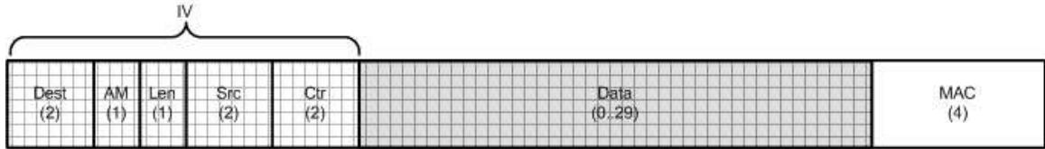
Figure 7: TinySec Packet Structure
