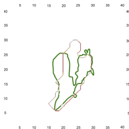
(b) Colina fire simulated using fast marching method compared to the actual Colina fire.
