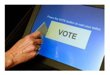
FIGURE 2 THIS IS AN EXAMPLE OF A NEWER DRE MACHINE. THE INTERFACE IS NOW  ${\sf GRAPHIC\ AND\ IS\ TOUCHSCREEN.}^{31}$
