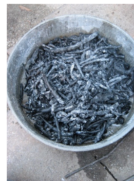
Figure 31. Biochar yield after cooking in an Estufa Finca stove.
