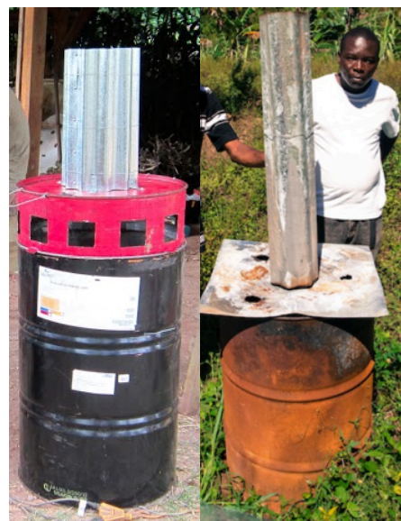
Figure 17 (right): A TLUD oven used in the Haiti case study project.
