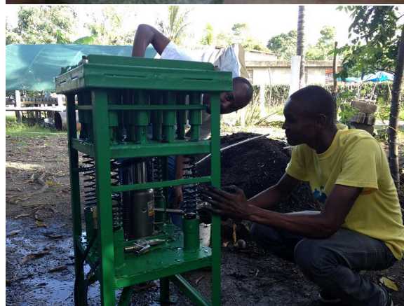
Figure 19 (top). A mechanical hand tool can create briquettes.
