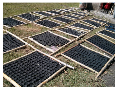
Figure 27. Green charcoal briquettes are laid out to dry at CRI’s production center.
