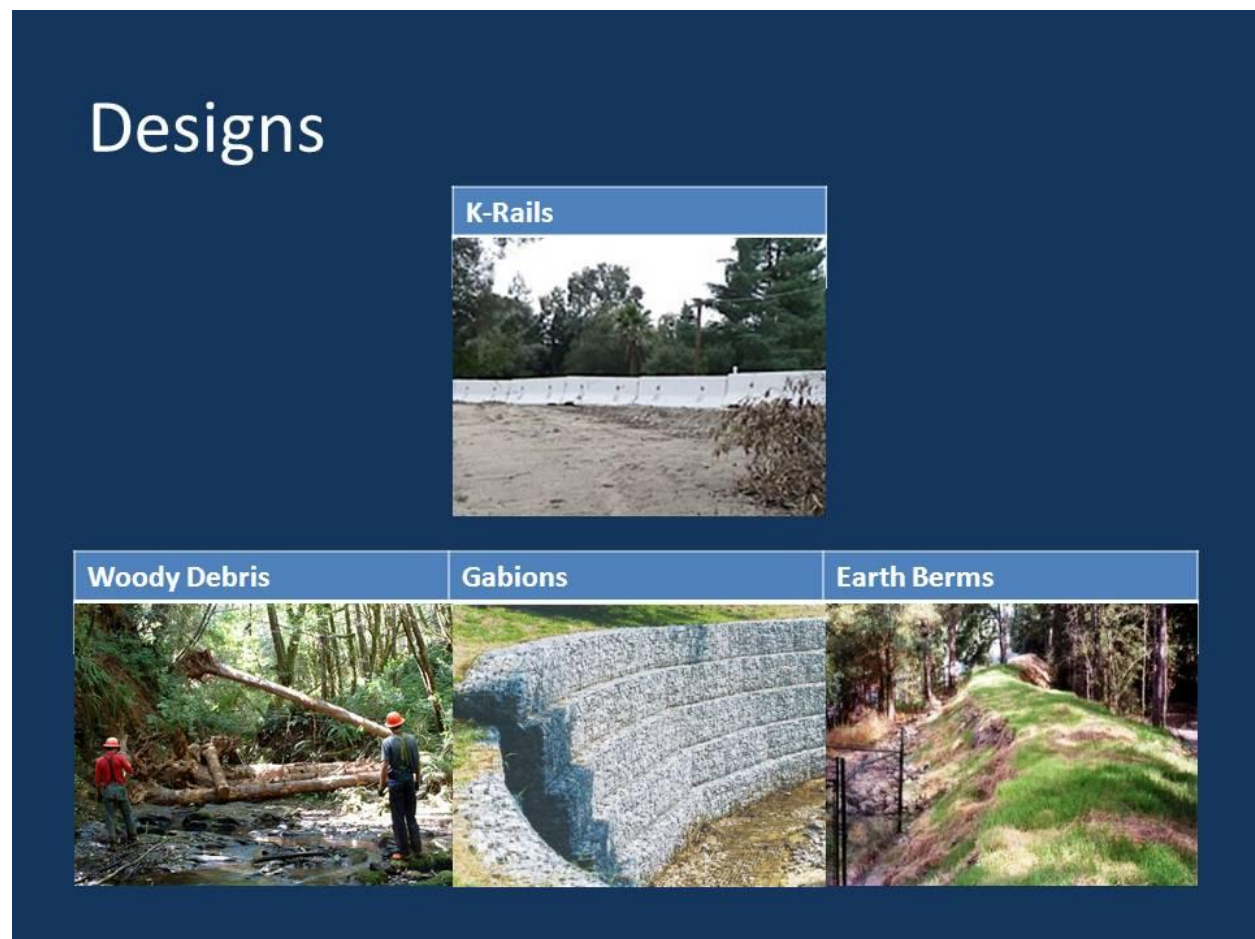
Figure 4. Alternative designs for the K-Rail replacement.
