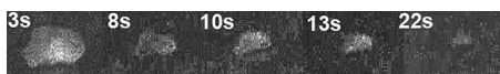
FIG. 2. The evolution with time of a hole (brighter area), or 2D polymer gas, within a polymer liquid (darker area) monolayer. The images are taken by Brewster angle microscopy (BAM). Variations in the beam intensity are off the same order of magnitude as the contrast for these two very thin films. Contrast has been improved with Photoshop™. Each image is 0.27 \text{ mm} \times 0.44 \text{ mm} .
