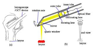
**Fig. 1** (a) Side view of the throat and larynx and (b) diagrammatic sketch of the laryngeal OCT sampling probe.
