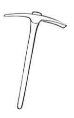
The pick mattock (similar to a pickaxe) is a very useful but potentially dangerous tool. To properly use it, grip the handle with your left hand at the bottom and your right hand at the top. Raise the tool over your right shoulder and as you swing it down, slide your right hand down until it hits your left. This tool is effective at removing hard rocks and breaking through cemented soil.
