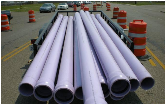
Purple pipes destined for non-potable water transport. Photo courtesy of HDR, Inc.
