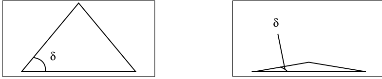
Fig. B.2 Left: Large angle of repose. Right: Small angle of repose.
