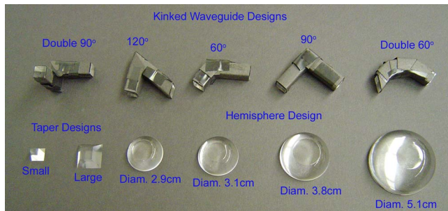
FIG. 8. (Color online) The photo shows many of the link designs that were fabricated and tested. Each design was created from a single piece of acrylic.
