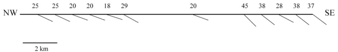
Figure 19: Cross Section of Cardiff Dome Perpendicular to Dominant Foliation. This cross section is 17 km long, and shows average foliation dips for every 1 km. In regions with no dip information there were no foliations dipping in the orientation of the cross section.
