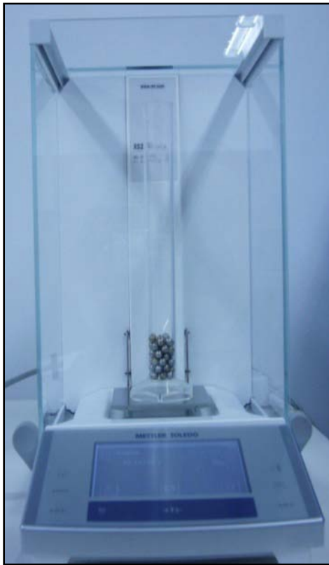
Figure 2. 2:( a) Determination of the weight of alum (b) Determination of the weight of Nylon
