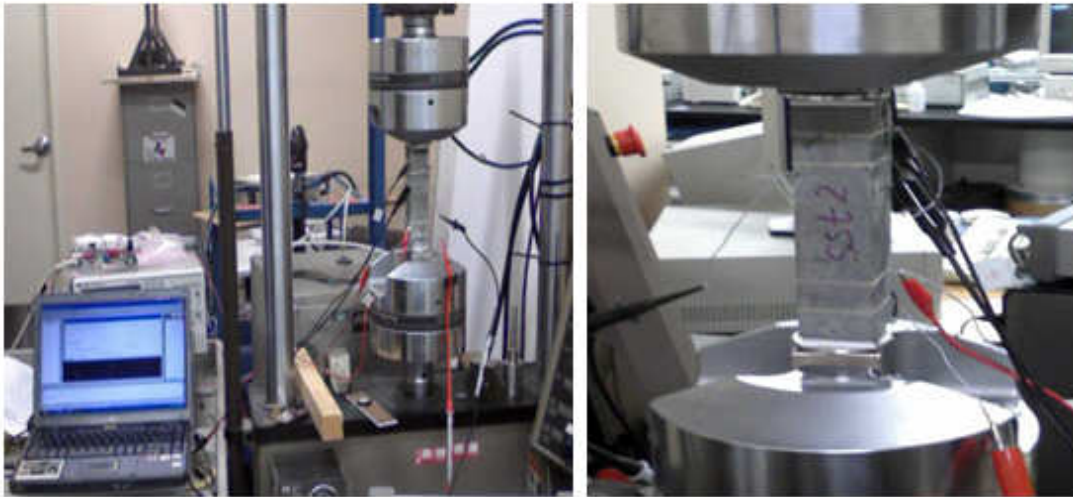
Figure 14: Smart concrete resistant measurement using MTS axial loading effect.
