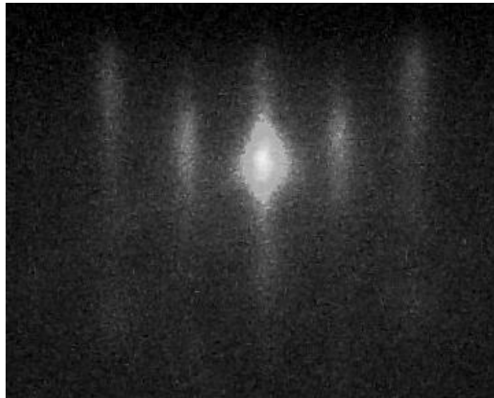
Figure 3.6. 2x1 reconstructed Si buffer layer.
