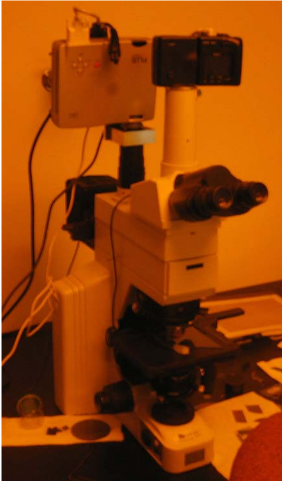
Figure 2.1: Our maskless lithography system. The projection lens of the DLP projector has been reversed and then mounted onto the microscope so that the image is projected into the focal plane of the microscope. Notice the amber overhead lights.
