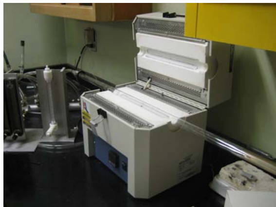
Figure 4.4: This furnace is normally used in the growth of nanotubes. It is capable of reaching over 1100°C, which is well above the temperature at which the graphite we use combusts.
