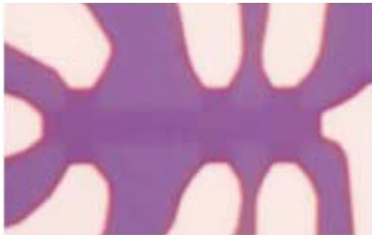
(a) This is a graphene Hall cross on 300\text{nm} of \text{SiO}_2 . Each terminal is connected to a gold electrode. This image is taken from Novoselov's paper on the room temperature observation of the quantum Hall effect[5]
