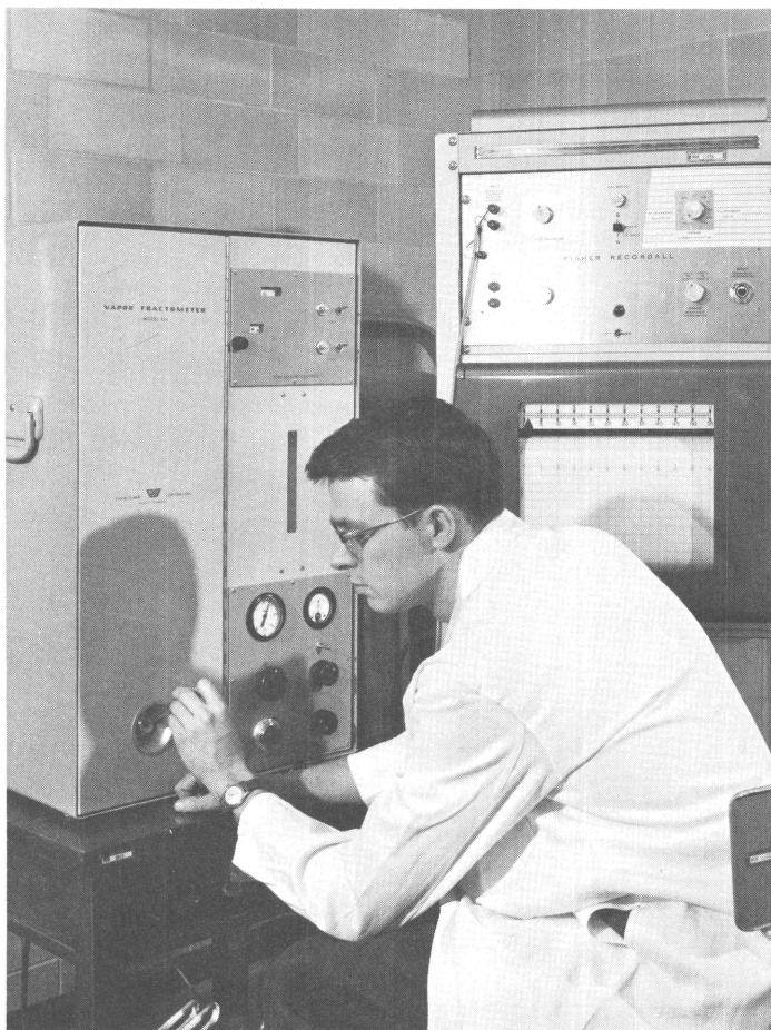
FIGURE 10.—Separation and Analysis of Low-Boiling Tar Acids Using Gas-Liquid Chromatography.
