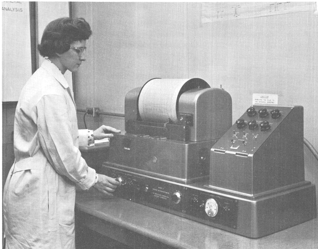
FIGURE 5.—Identification and Analysis of Tar Acids and Bases With an Infrared Recording Spectrophotometer.
