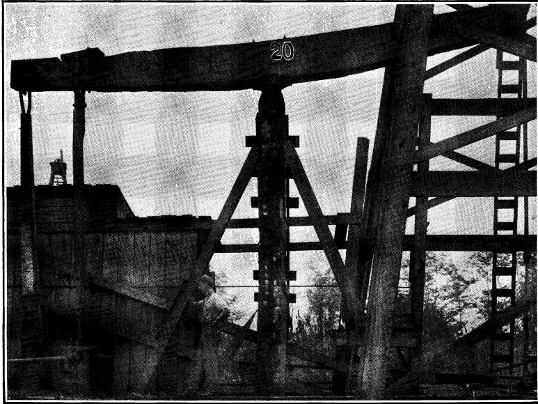
A. OIL WELL FROM WHICH CASING HEAD GAS IS DRAWN FOR NEAR-BY GASOLINE PLANT.
