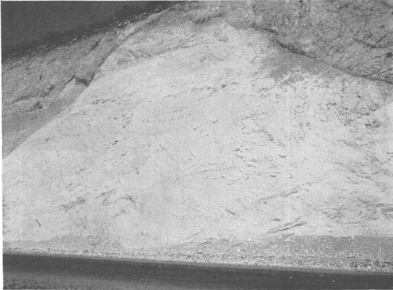
FIGURE 16.—Oregon 5 deposit, Harney County. Dark areas are clayey soil. Note gravel at top left.
