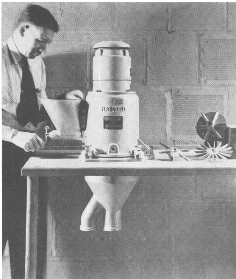
FIGURE 29.—Laboratory-size air separator. The small fan and the 6- and 16-bladed whizzers are shown at the right. When the separator is used, cloth bags are clamped onto the two spigots—the larger spigot for the fine product, and the smaller for the oversize product.
