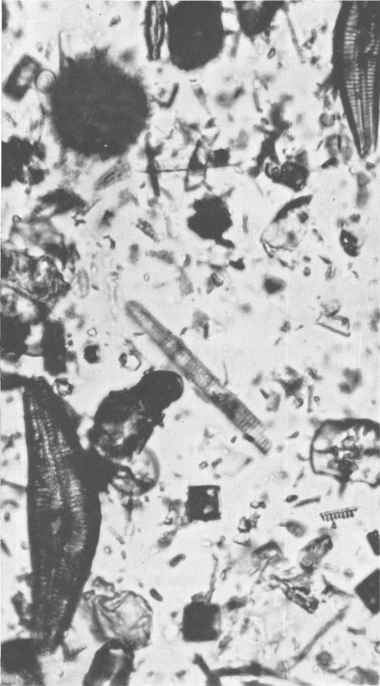
FIGURE 36.—Photomicrograph of diatoms and diatom fragments in the slow flow-rate filter-aid made from 250- to 325-mesh diatomite from Big Lake, Wash. (Washington 17). \times 1,000 . Clear, semi-rounded particles in lower half are quartz grains.
