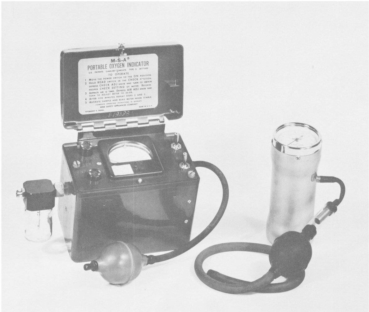
FIGURE 53.—Portable Oxygen Indicator and Quick-Check Analyzer.
